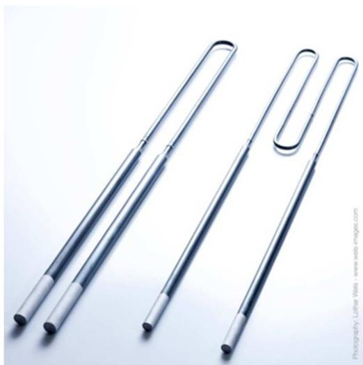
**MolyCom®-Ultra and MolyCom®-Hyper** electric heating elements are metallic-ceramic materials mainly composed of molybdenum disilicide ( $\text{MoSi}_2$ ). Above 1000 °C (1832 °F) service temperature the surface will form a protective high temperature layer of pure quartz, which gives the MolyCom®-Ultra and MolyCom®-Hyper material a high resistance to oxidation.
